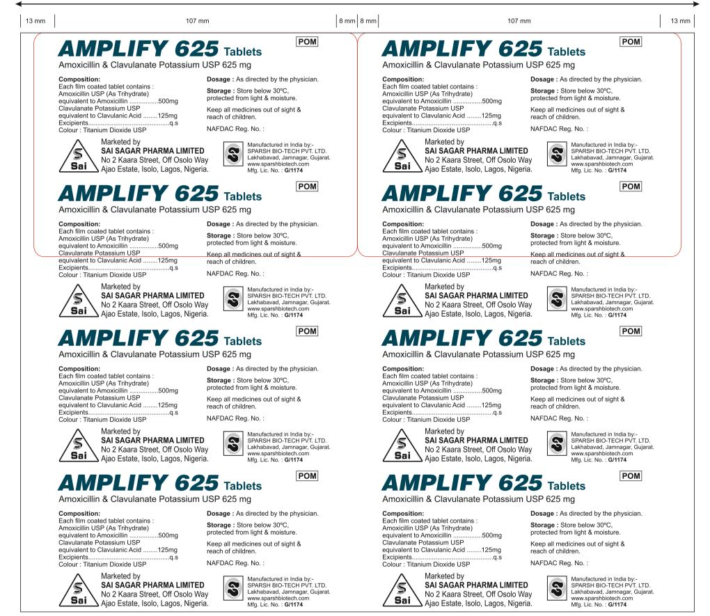
Foild Width : 256 mm Bister Size : 123 x 85 mm Repeat Length : 55 mm Colour : Pantone 548 C, Black Thickness : 0.04
